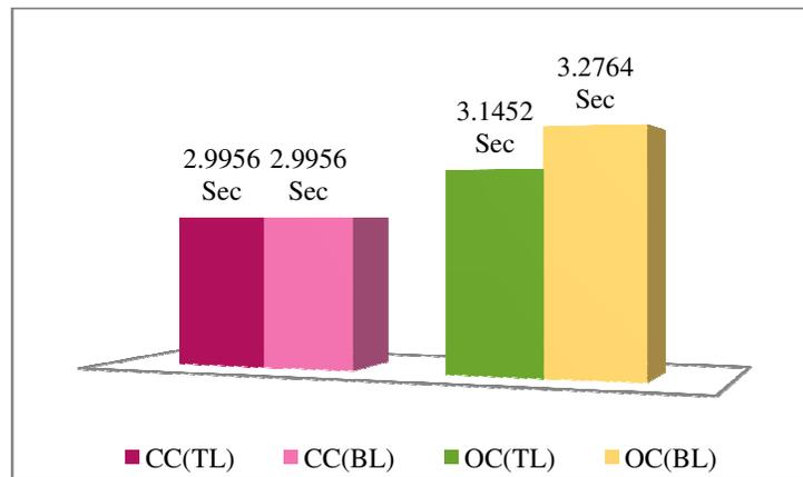
Table 4 and Figure B showed the wetting time in seconds for both CC and OC samples. The wetting time for CC was less for both top and bottom layers than OC. The wetting time recorded for CC(TL) was 2.9956 seconds and the same was observed for CC(BL). Whereas, the wetting time of OC(TL) was 3.1452 seconds and 3.2764 seconds OC(BL). According to the T-value of the two samples compared, there was no significant difference in the wetting time of CC and OC samples on both top and bottom layers.
