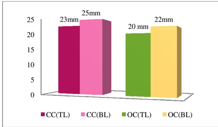
Table 6 and Figure D showed the maximum wetted radius of CC and OC samples. The maximum wetted radius for CC was observed to be more in both top and bottom layers than for OC. The maximum wetted radius for CC(TL) was 23mm and for OC(TL) was 20mm. The maximum wetted radius for CC(BL) was 25mm and that for OC(BL) was 22mm. The T-values show a significant difference in the maximum wetted radius of CC and OC samples on both top and bottom layers.
