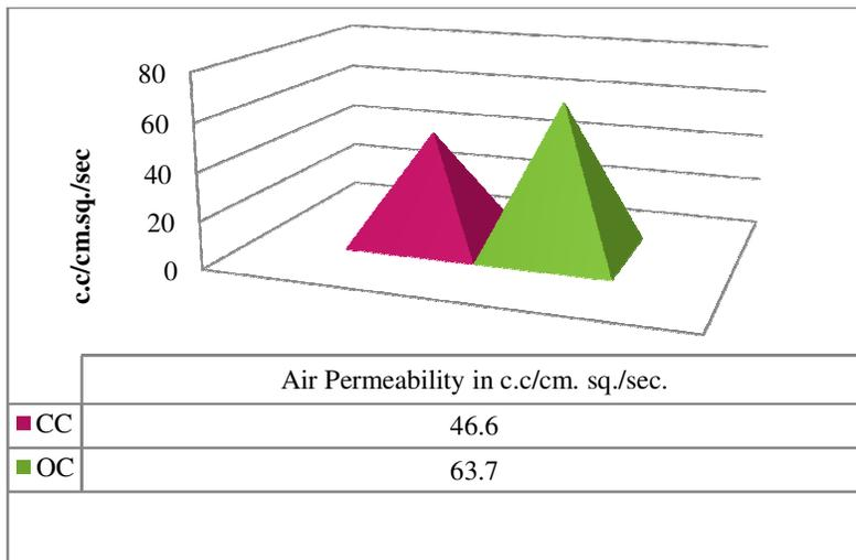
Table 3 and Figure A showed the air permeability for CC and OC samples. The air permeability for CC was less than that of OC samples. CC recorded the air permeability of 46.6 c.c/cm.sq/sec. whereas OC samples recorded air permeability of 63.7 c.c/cm.sq/sec. According to the T-value of the two samples compared, there was a significant difference in the air permeability of CC and OC samples.
