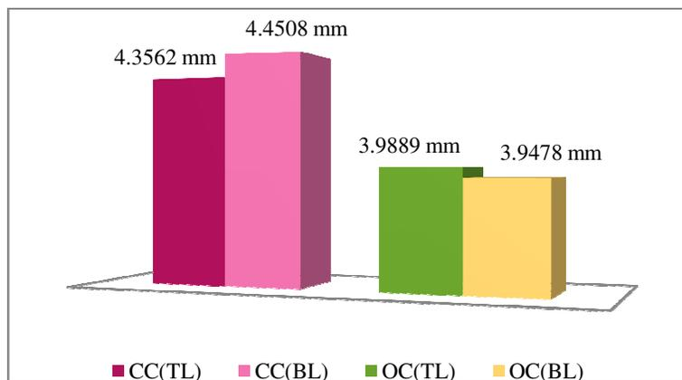
Table 7 and Figure E showed the spreading speed in mm/sec for CC and OC samples. The spreading speed was faster for CC samples than for OC on both top and bottom layers. The spreading speed for CC(TL) was 4.3562 mm/sec whereas for OC(TL) it was 3.9889 mm/sec. The spreading speed for CC(BL) was 4.4508 mm/sec and that for OC(BL) was 3.9478 mm/sec. The T-values show a significant difference in the spreading speed of CC and OC samples on both top and bottom layers.
