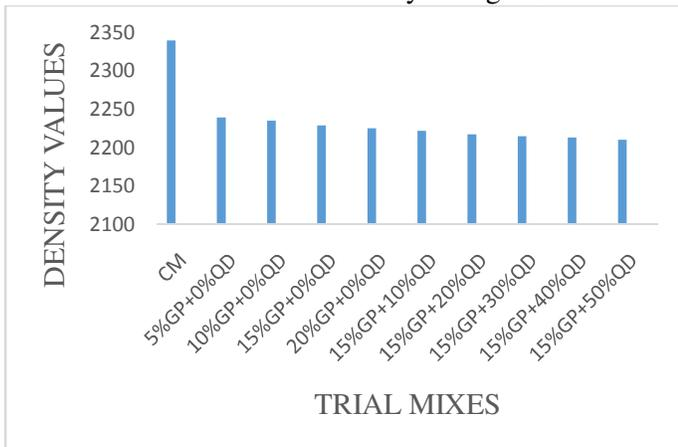
Figure 4.9 Density value of various trial mixes for 7 days
