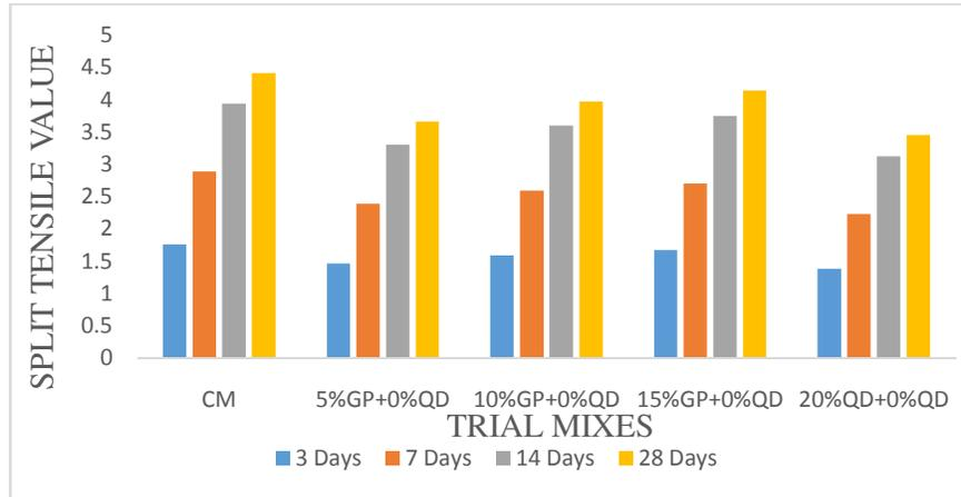
Figure 4.5 Impact of partial replacement of cement by glass powder on split tensile value of cylinder
