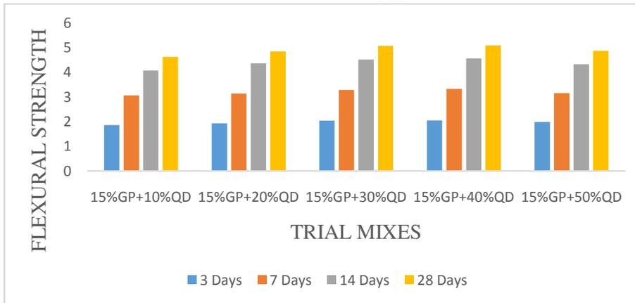
Figure 4.8 Impact of partial replacement of cement by glass powder and fine aggregate by quarry dust on flexural strength of beam
