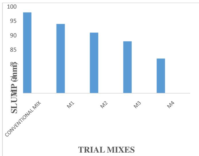
Figure 4.1 Slump test values for trial mixes with partial replacement of cement by glass powder
