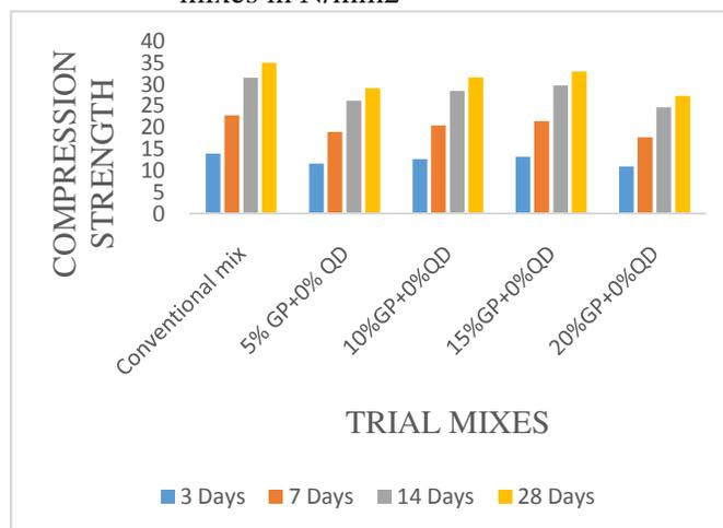
Figure 4.3 Impact of partial replacement of cement by glass powder on compression value of the cube
