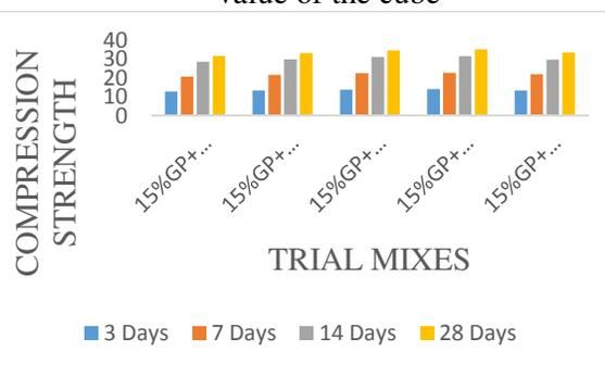
Figure 4.4 Impact of partial replacement of cement by glass powder and fine aggregate by quarry dust on the compression strength of cube.
