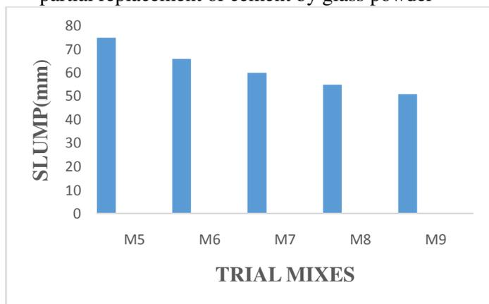
Figure 4.2 Slump test values for trial mix with partial replacement of cement by glass powder and fine aggregate by quarry dust
