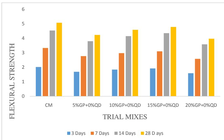
Figure 4.7 Impact of partial substitution of cement by glass powder on flexural strength of beam
