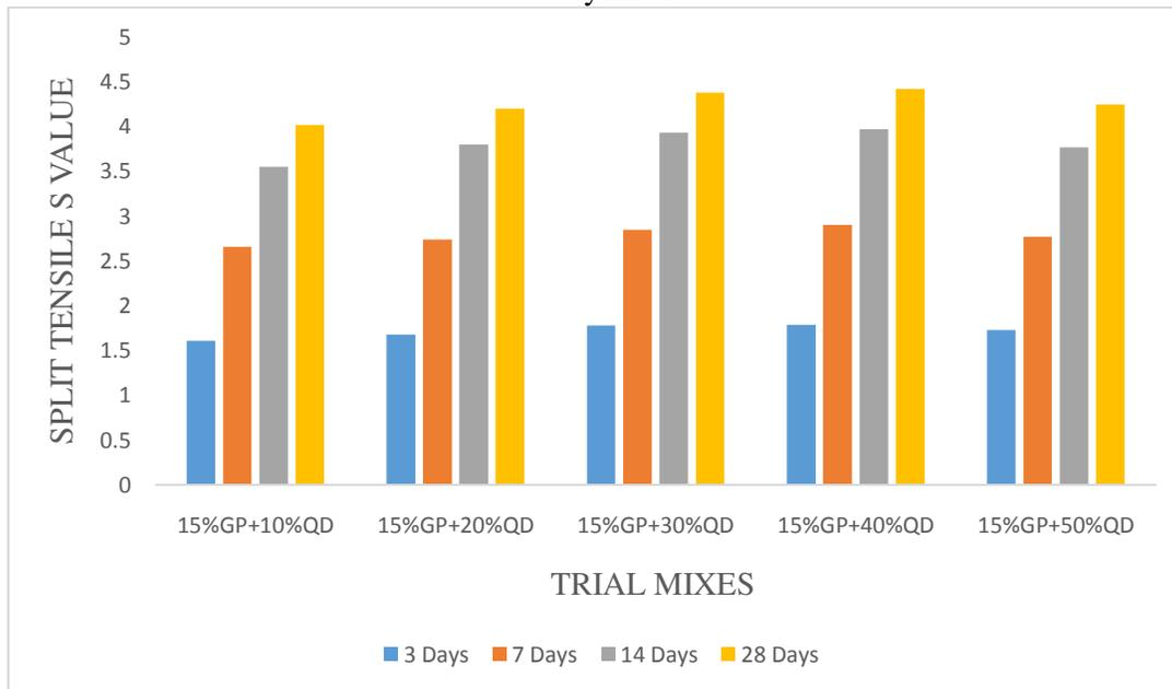
Figure 4.6 Impact of partial replacement of cement by glass powder and fine aggregate by quarry dust on split tensile strength of cylinder
