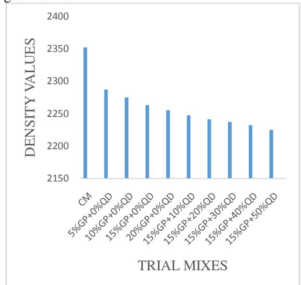
Figure 4.10 Density value of various trial mixes for 28 days
