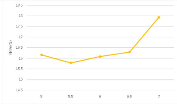
**Figure No:4.5 Voids in Mineral Aggregate v/s bitumen content**
