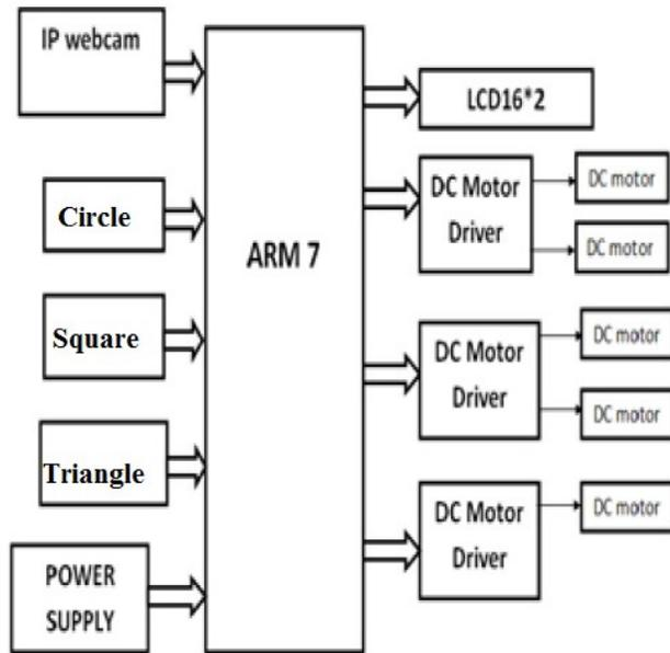
Fig.1 Block diagram of praposed system
