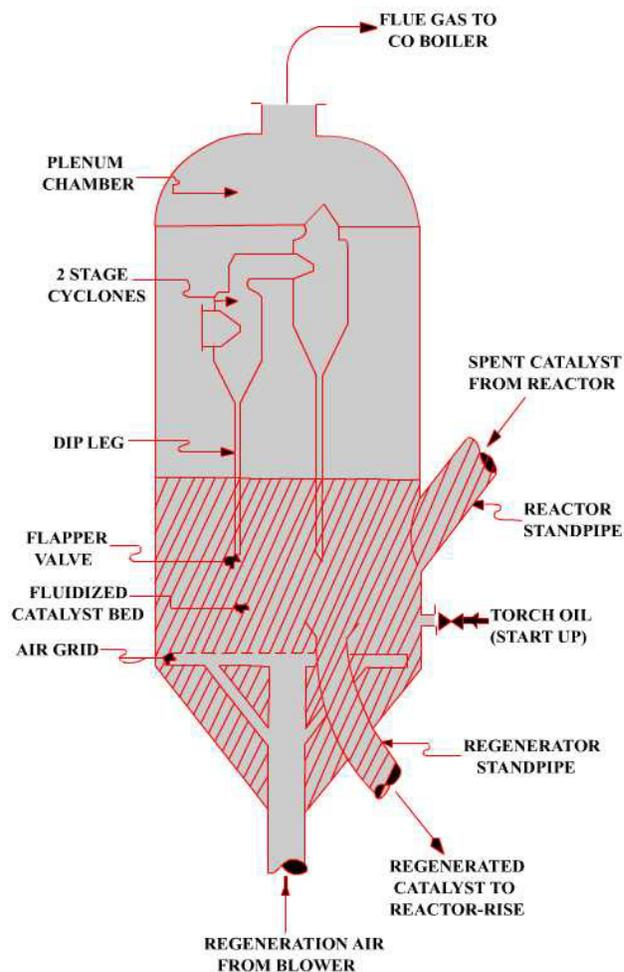
Figure 1: Schematic of FCCU Regenerator
