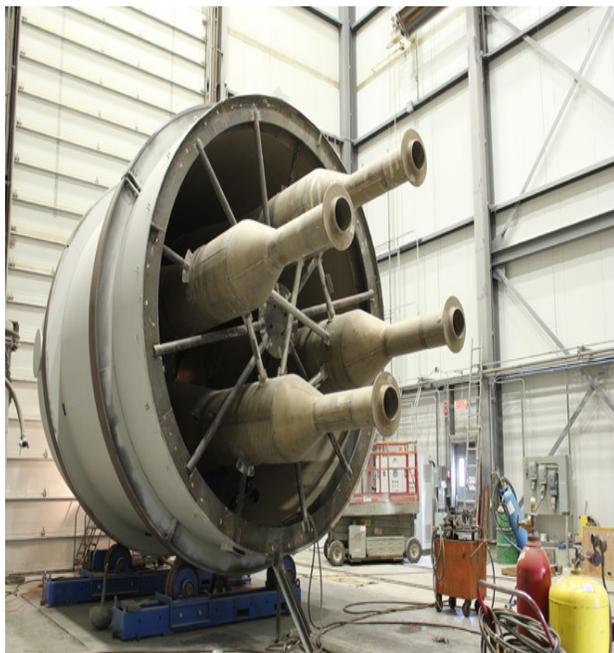
Figure 2: Regenerator cyclone separators
