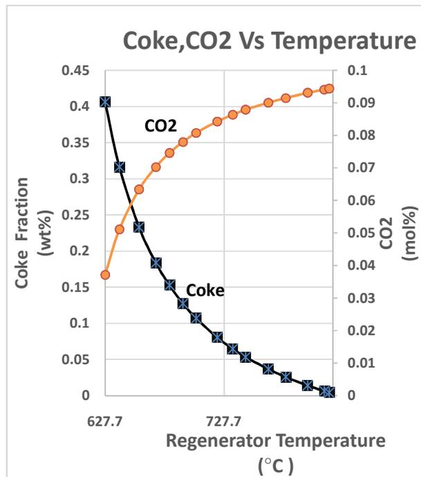
Figure 5: Effect of Temperature and CO<sub>2</sub> mole fraction on Coke.
