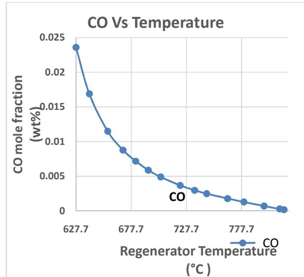
Figure 4: Effect of Temperature and CO mole fraction.
