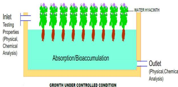
Fig 1 Representation of Experimental Model
