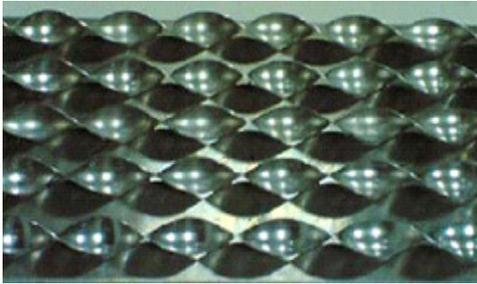
**Figure 4.1 Multiple Twisted Tape**
