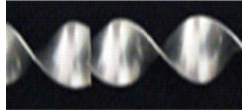
**Figure 3.1 Alternate Clockwise and Counter-Clockwise Twisted-Tapes**
