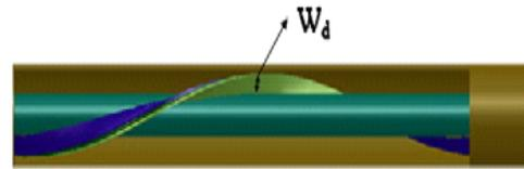
**Figure 5.1 Test Section Fitted with Triple Helical Tape Insert with a Core-Rod**
