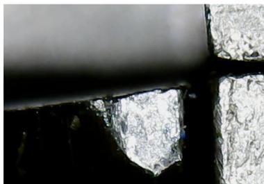
Top view of tool after machining
