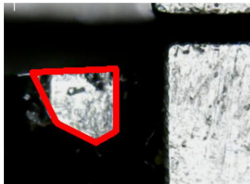
Front View of Tool wore after machining
