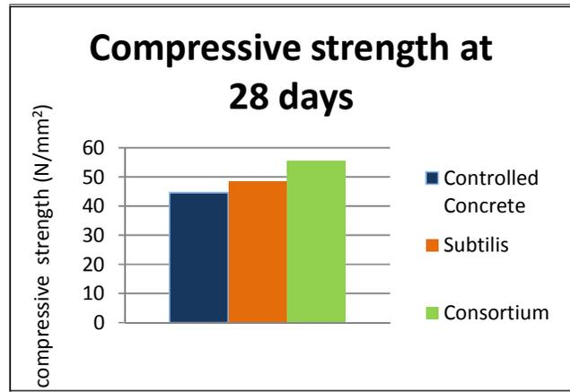
Fig. 3 Compressive strength at 28 days of curing
