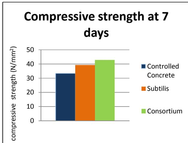
Fig. 2 Compressive strength at 7 days of curing
