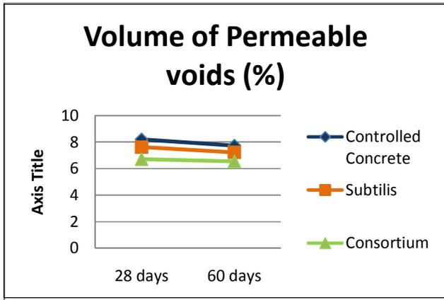
Fig. 7 Volume of Permeable voids in different concrete specimens
