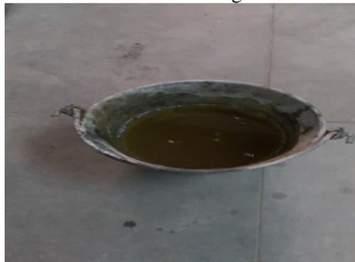
Fig. 1 Bacterial solution prepared to be added in concrete
