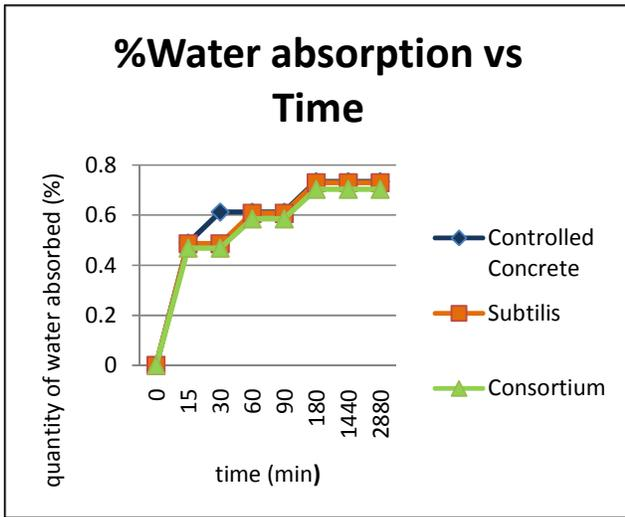
Fig. 4 Water absorption vs. time Graph
