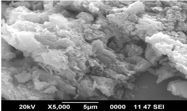
Fig. 9 SEM images of controlled concrete demonstrating more voids
