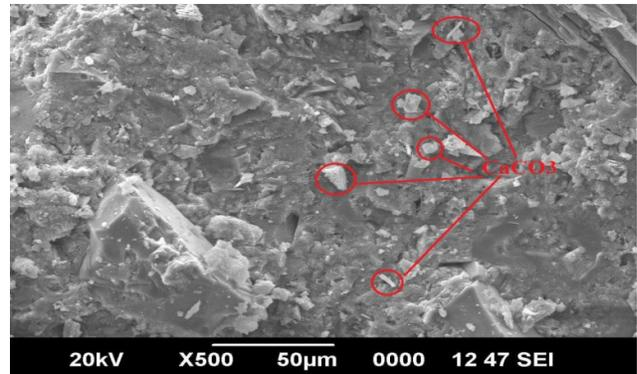
Fig. 11 Image of Concrete with Bacillus Subtilis showing clustered lamellar of CaCO<sub>3</sub>
