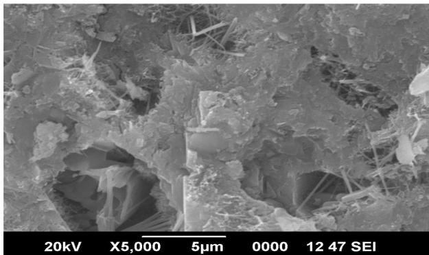
Fig. 10 SEM image of Bacterial concrete showing a denser microstructure
