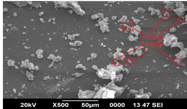
Fig. 12 Image of Concrete with consortium of bacteria showing CaCO<sub>3</sub> crystals
