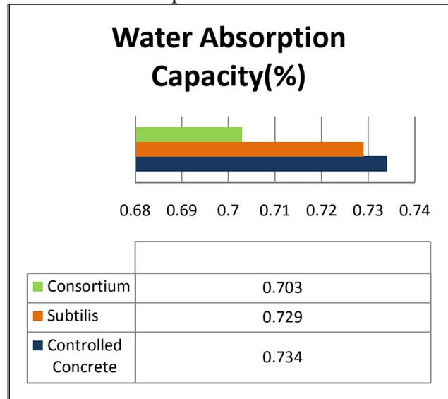
Fig. 5 Water Absorption Capacity in % for different concrete specimens
