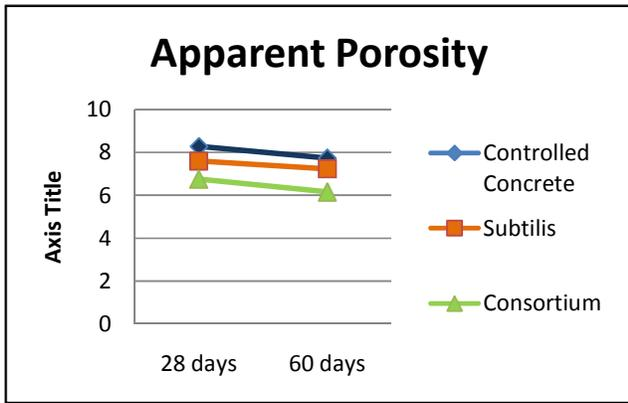
Fig. 6 Apparent Porosity of different concrete specimens
