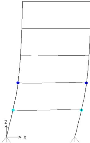
FIGURE 8. IMMEDIATE OCCUPANCY LEVEL FOR 5 STOREYS
