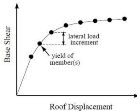
FIGURE 1. CAPACITY (PUSHOVER) CURVE OF STRUCTURE
