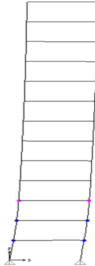
FIGURE 9. IMMEDIATE OCCUPANCY AND LIFE SAFETY LEVEL FOR 13 STOREYS
