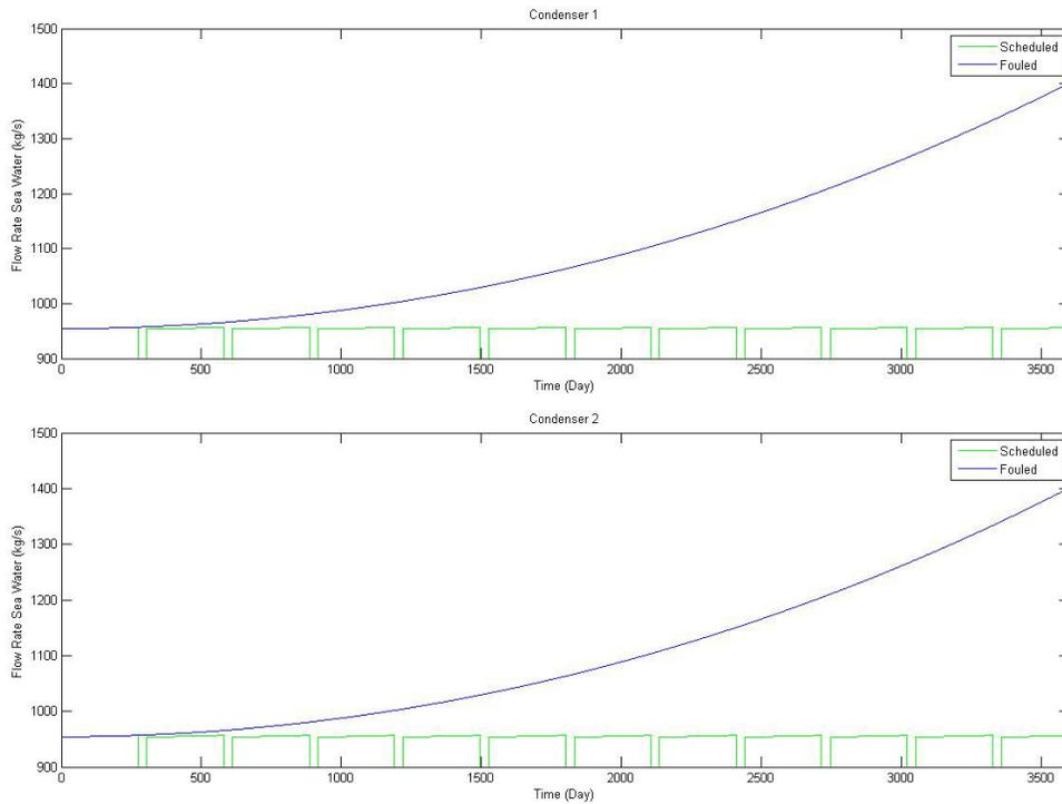
Fig. 3 Flow Rate Sea Water under Fouled and Cleaning Scheduled
