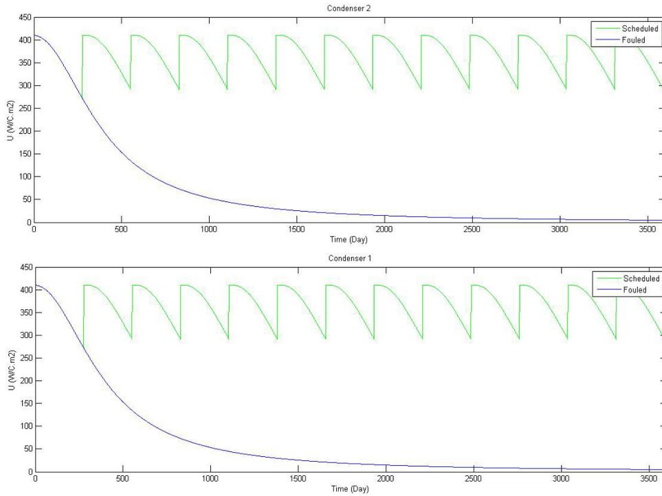
Fig. 2 Overall Heat Transfer under Fouled and Cleaning Scheduled
