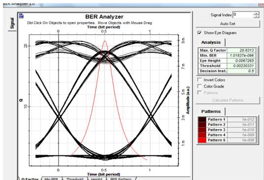
Fig 9 Eye diagram of Gaussian pulse uniform fbG raised cosine filter
