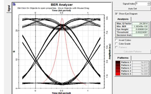
Fig 8 Eye diagram of Gaussian pulse uniform cosine roll off filter
