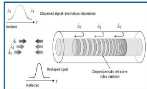
Fig 1 FBG compensate for dispersion by reflecting different wavelengths at different locations along the grating lengths
