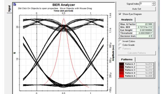
Fig 7 Eye diagram of Gaussian pulse fbg raised cosine filter
