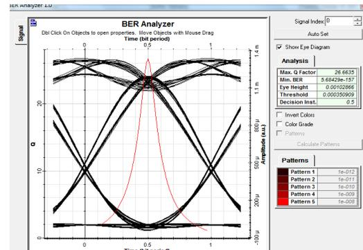
Fig 6 Eye diagram of Gaussian pulse fbg cosine roll off filter
