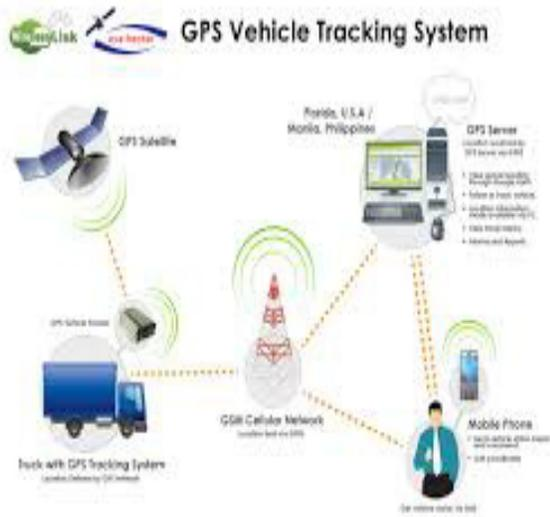
Fig1.GPS System Architecture
