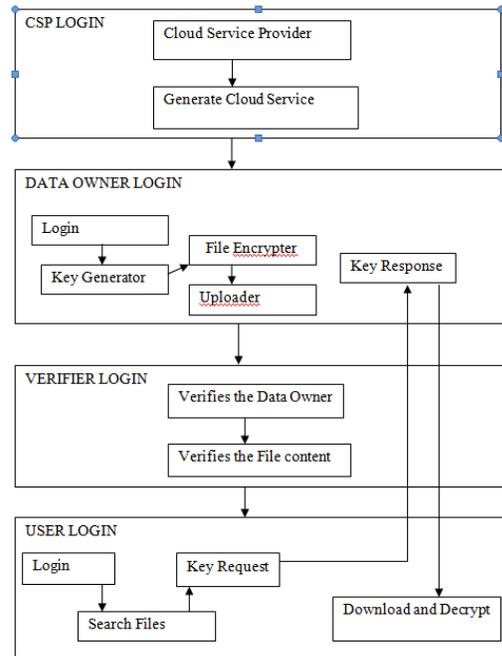
CSP generates cloud servers for the number of users. Data Owner login and key is generated for the file, to be encrypted. Then the encrypted file is uploading to the cloud for the interested users. Verifier verifies the file and generated signature. User login, search the file and request for the key to the Data Owner. Data Owner response for the key request. Data Owner sends the key response to the User Login. User Login decrypt and download the file.
