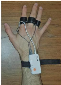
Fig5 Proposed system transformed into a wearable device
