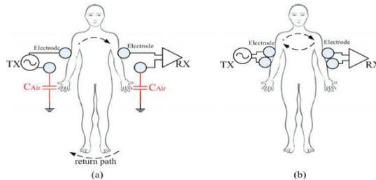
Fig.2 Capacitive coupling
