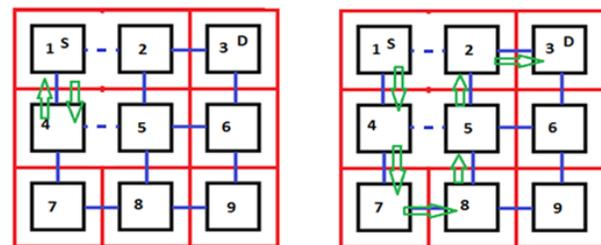
(a) Deadlock (Conventional XY-Routing algorithm) (b) No deadlock (Proposed XY-Cruise algorithm)
