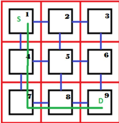
Fig. 3 A 3x3 Mesh Network with dataflow from (1,1) to (3,3) (Case 1)
