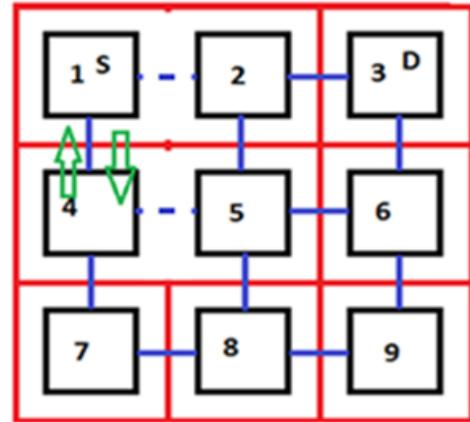
Fig. 2 A 3x3 mesh network with deadlock between routers 1 and 4.
