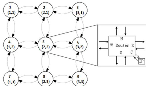
Fig. 1 A 2 dimensional 3x3 Network-on-Chip (NoC) with the mesh topology.
