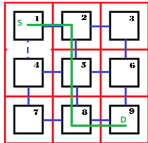
Fig. 4 A 3x3 Mesh Network with dataflow from (1,1) to (3,3) with a single fault (Case 2)
