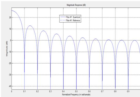
Fig.8 Filter response of CIC Interpolator
