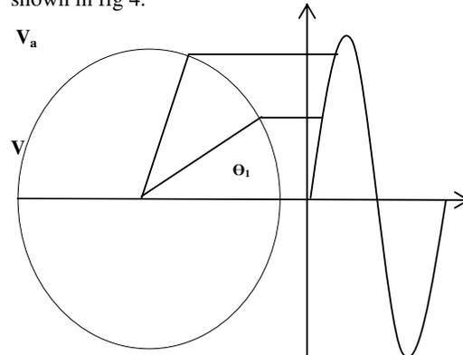
Fig.4 Operation of the phase accumulator in a DDS
