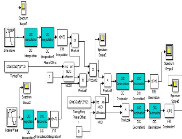
Fig.7 Simulink model of a WiMAX system
