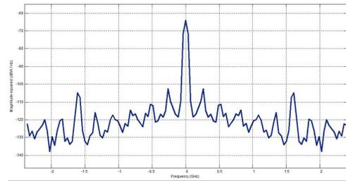
Fig.12 Output signal of DUC
