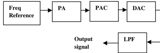
Fig.3 Block diagram of DDS
