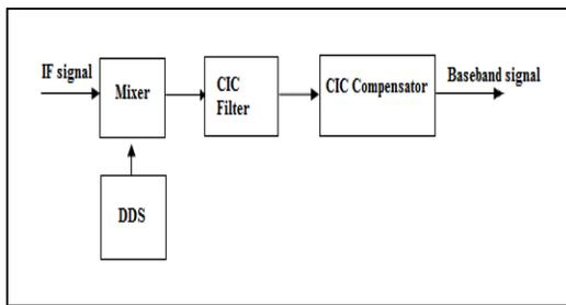
Fig. 2 Block diagram of Digital down converter
