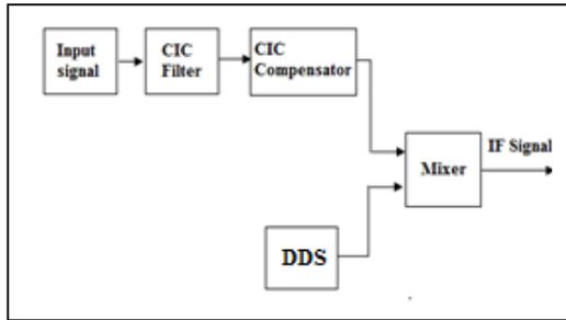
Fig 1 Block diagram of Digital up converter
