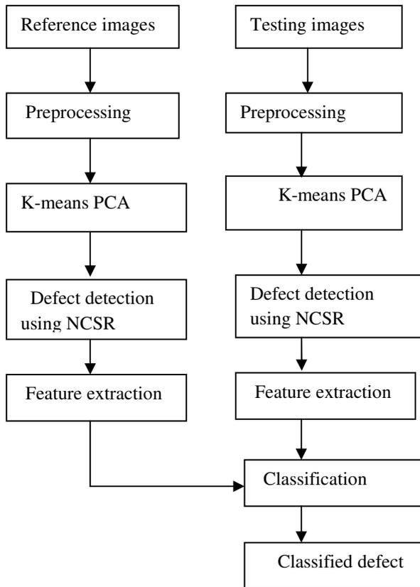
Fig.1. Flowchart of the defect detection process includes dictionary learning and detection model
