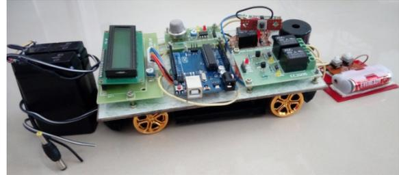
Fig. 3 Hardware for transmitter and receiver module
